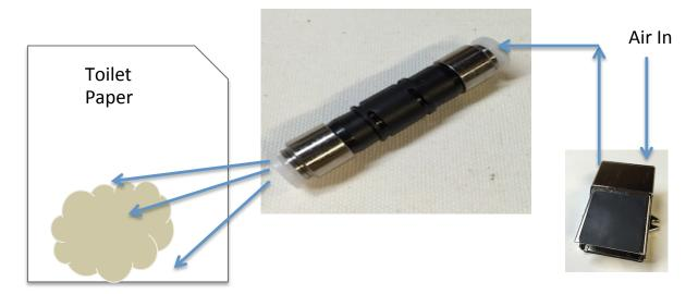
With the output hose removed apply air to the machine and force the air into a piece of toilet paper. Check for dirt, debris, oil and moisture. In most cases this will clean out the quick exhaust, if this does not resolve the problem than purchase a Quick Exhaust here: <a href="https://gallerystretcher.com/product/quick-exhaust/">https://gallerystretcher.com/product/quick-exhaust/</a>
