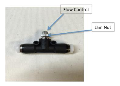
If the Clamping Bar is still moving sluggishly after cleaning then loosen the jam nut by turning it counter-clockwise as viewed from the top. Then turn the flow control knob counter-clockwise about ½ turn. Test the Clamping Bar and if that solves the problem retighten the jam nut.
