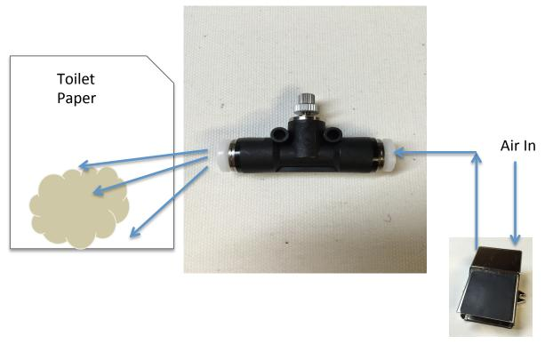
With the output hose removed apply air to the machine and force the air into a piece of toilet paper. Check for dirt, debris, oil and moisture. In most cases this will clean out the Flow Control.
