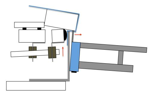
The "clamp bar" will tend to rise during a stretch because we are exerting a tremendous amount of upward force during a stretch. The amount that it rises depends on a number of variables mentioned below. As long as the 'clamp bar" drops back down after a stretch than it is working correctly.
